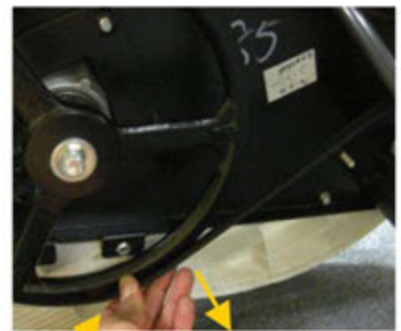
3. Remove the drive belt by pulling down on the belt while spinning the large pulley to un-wind the belt off.
