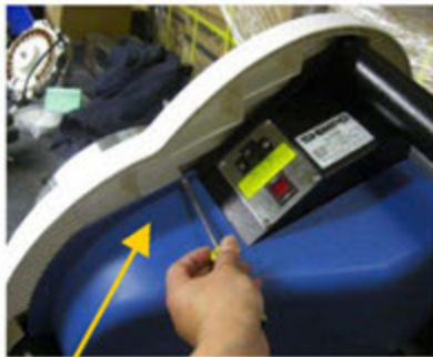
1. Remove the undercover by removing all undercover screws.
