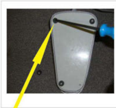
1. Unscrew the 4 feet using the Phillips screwdriver
