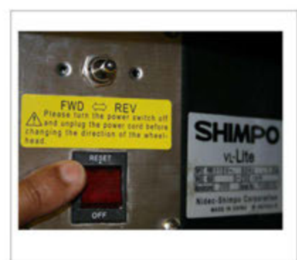
6. Make sure the foot pedal is in the STOP position. Turn the power ON and follow the Resetting the Potentiometer guide.
