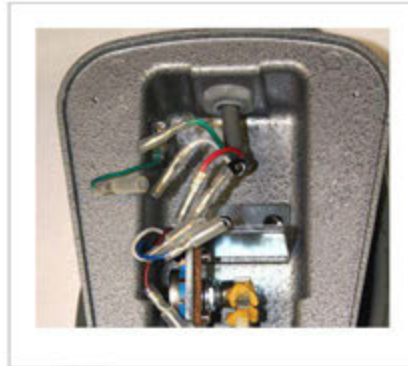
2. Remove the cover and unplug all 3 wires from the potentiometer.
