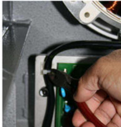
2. Cut the zip tie to release cables that are zip tied together.
