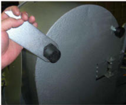
1. Remove the four feet off bottom of the wheel using the RK-Wrench (spanner). Then remove the metal cover plate.
