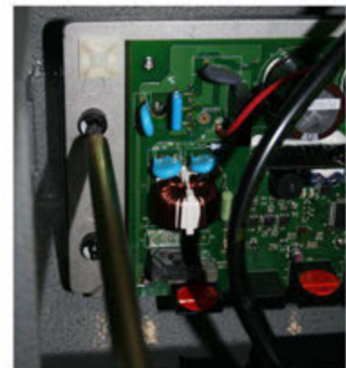
6. Unscrew the 4 mounting bolts as well as the green ground wire to take off the controller.
