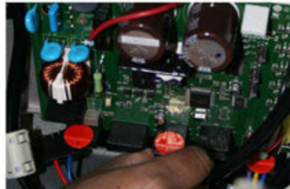
5. Un-clip all 5 cables from the control board by squeezing the sides of the clip and pulling.
